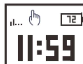
6) Battery Status: The battery icon shows the percentage value of the remaining battery level. The lightning symbol “⚡” is shown when charging and the percentage value is updated in real time. When the battery is fully charged, the battery icon will show “100”, as shown in the figure below:
