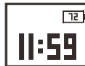
2) Wireless Presenter Disconnected Status: When the wireless presenter has been connected normally, if you unplug the USB receiver or turn off the Bluetooth of your computer, the display of the wireless presenter will show the disconnected status, as shown in the figure below:
